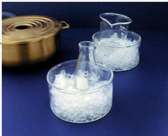
You can now place the flask in an ice bath to finish the crystallization process.
