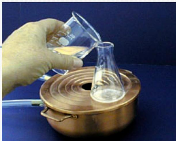
Pour a small amount of the hot solvent into the flask containing the solid.
